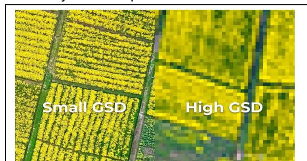
1. How many data measurements (ground squares or pixels on above right figure) on the ground for an image with GSD = 0.25 feet would fit in a 10 ft by 10 ft area on the ground?
