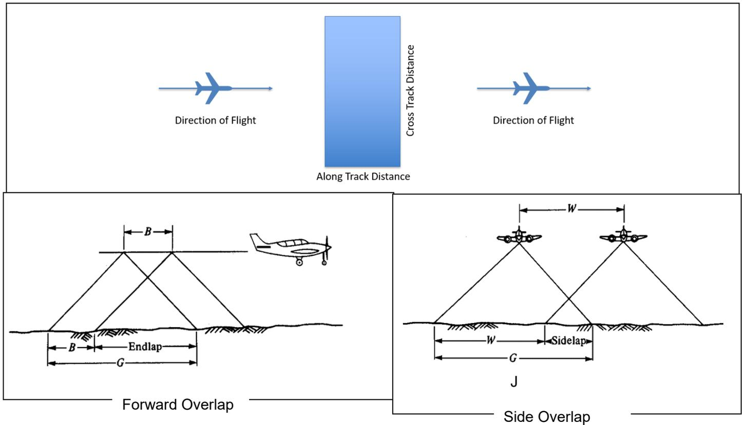
7. Using a GSD = 0.5 feet, find the along track distance (G), the cross-track distance (J), the travel distance between consecutive collected photographs (B), and the width distance between flight lines (W) for each camera below. Extend the table below to include the four additional columns.
