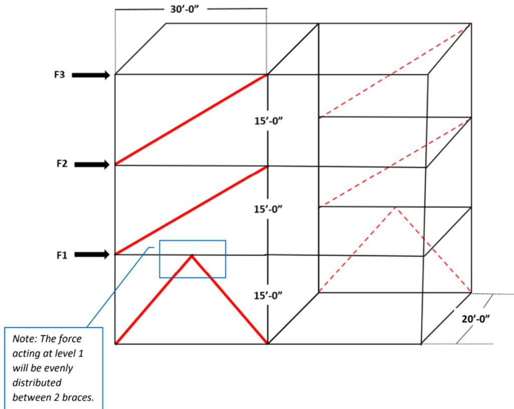
1. Each diagonal brace must support the sum of all lateral forces at or above the brace; for example, the total force acting on  $F_2$  must also include the force acting on  $F_3$ . What would be the lateral force, measured in kips, exerted at each level?
