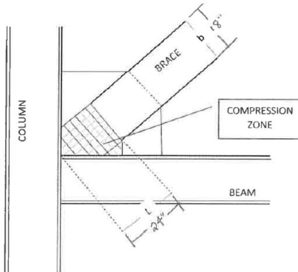
Euler’s equation helps us determine the maximum compression for various plate thicknesses before buckling occurs. The equation we use to determine the critical buckling load is:
