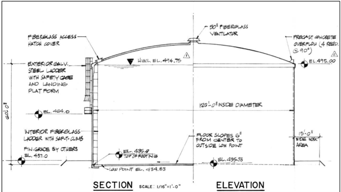
3. In addition to the weight of the water, we must also consider the weight of the empty concrete tank. The tank wall is 15 inches thick and the floor is 4 inches thick. The top of the tank is fiberglass and weighs 170,000 #.
