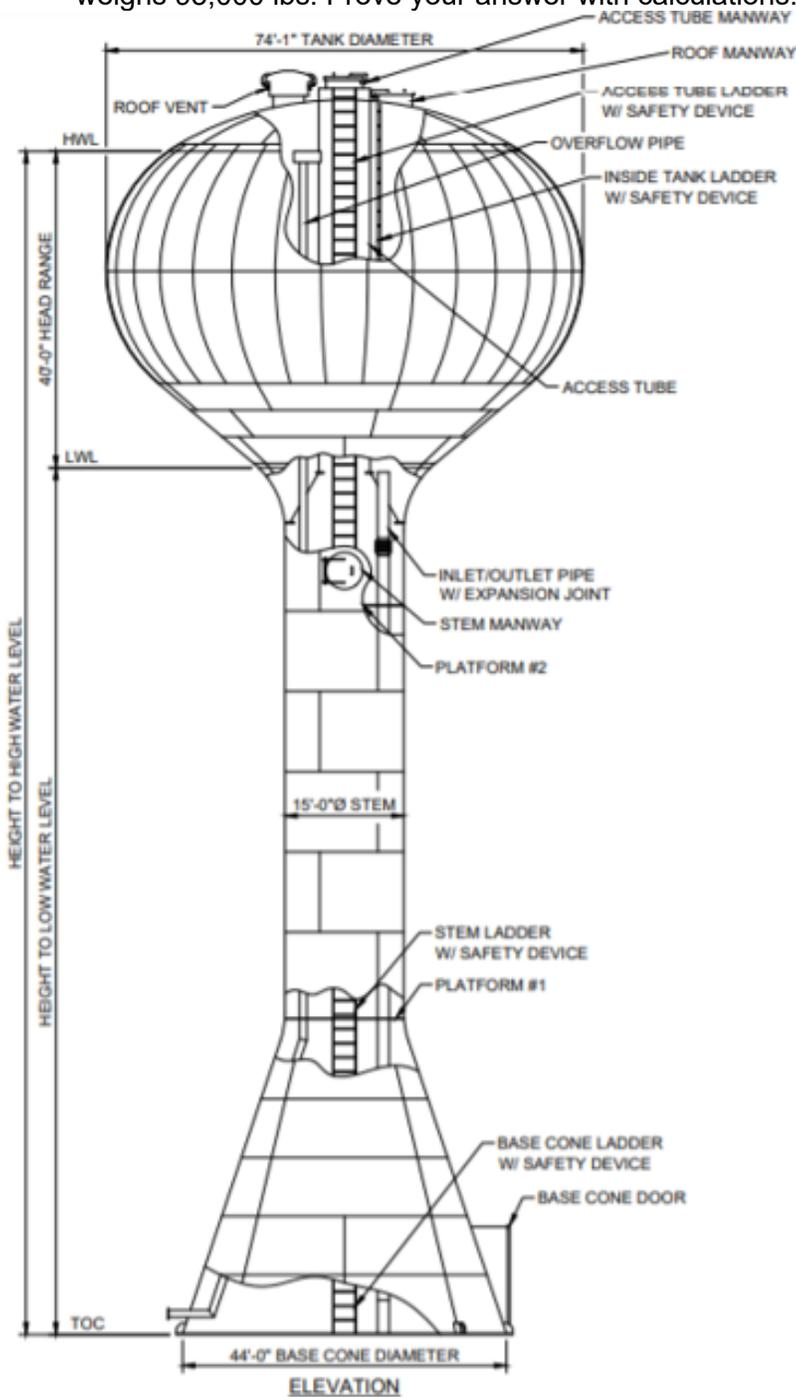
8. What is the maximum amount (volume) of water that this spherical steel tank can hold given the site for the water storage tank has very good soil and the dimensions of the water tower remain unchanged?
