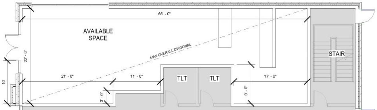
8. Suppose the developer decides to eliminate the planned sprinkler system in order to reduce costs. Identify the area of the building that is now “off limits” for the placement of a second exit to meet the code for assembly occupancy. Show the area that is off limits on the floor plan below. (Show work to justify your answer.)
