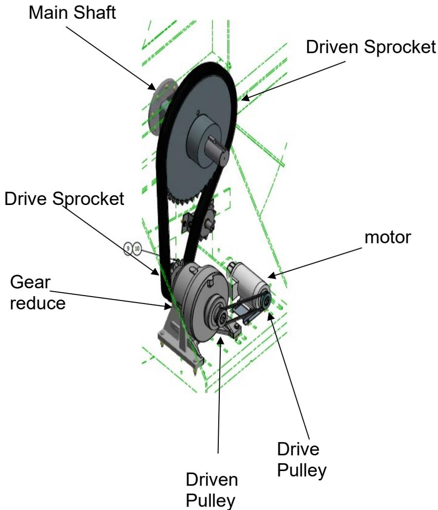
1. How many RPMs does the Driven Pulley rotate?
