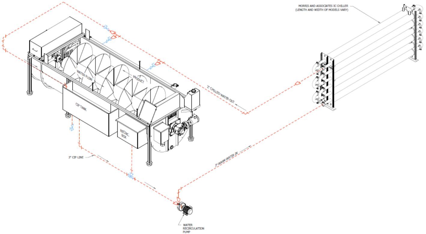
1. The CIP tank must be filled with enough hot soapy water to clean the entire run of tubing. Industry standard is to size the CIP tank at least 15% more than the volume of the tubing so that there will be some water left in the tank after the tubes are filled. What size CIP tank should you put on the machine?
