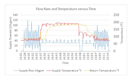
1. Supply water flow rate (gpm): This is a measurement of the flow rate of the water entering at the beginning of the circuit. It is important to note that the graph of this data shows 3 distinct sections that each pertain to one of the cleaning phases.
